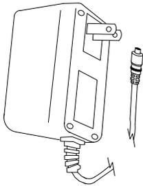
**ENGINEERING SPECIFICATION: P6900-PCF12 Plug-In Power Converter** – Plug-in Power Converter is designed to provide 12VDC power for one Zurn 12VDC sensor faucets. Power converter plugs into 120VAC outlet (supplied by others) located conveniently to faucets. Electrical characteristics: Input: 120VAC, 60Hz, 25w; Output: 12VDC, 800mA
