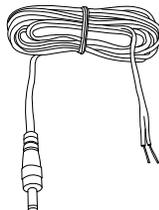
**ENGINEERING SPECIFICATION: Zurn P6900-CWB Connecting Wire –** Connecting wire to convert/connect battery-operated sensor faucet to P6000-HW6 power converter. The connecting wire is 84" long with one end bare to connect to power converter and the opposite end has an RCA connector to plug into electronics module of the faucet.
