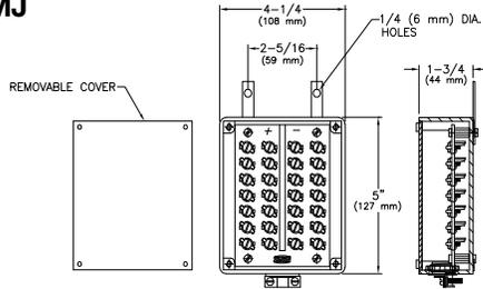
**ENGINEERING SPECIFICATION: ZURN P6000-MJ –** The Mini Junction Box is a 4-1/4" x 5" x 1-3/4" [108 mm x 127 mm x 44 mm] electrical enclosure designed to connect up to 8 Zurn sensor urinals/closets. The unit includes a high impact plastic enclosure with polarity marked terminal board, high impact plastic cover panel, wall mounting tabs, integral strain relief, and illustrative wiring diagram.
