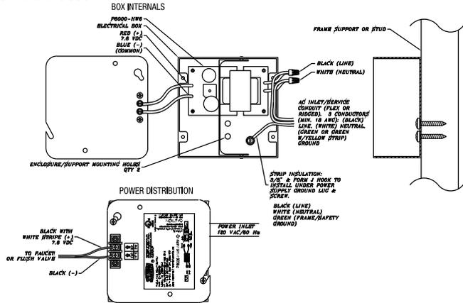
**ENGINEERING SPECIFICATION: Zurn P6000-HW6 Hardwired Power Converter –** Hardwired power converter to power up to 8 Zurn sensor urinal/closet flush valves or up to 8 hardwired Zurn sensor faucets. The P6000-HW6 is integrated within a 4-11/16" x 4-11/16" x 2-1/8" electrical and the low voltage connections are performed at the terminal block mounted externally on the box cover.
