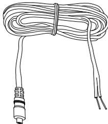
**ENGINEERING SPECIFICATION: Zurn P6900-CWE Connecting Wire** – Connecting wire to convert/connect sensor faucet to a 12VDC power converter. The connecting wire is 84" long with one end bare to connect to power converter and the opposite end has an RCA connector to plug into electronics module of the faucet.
