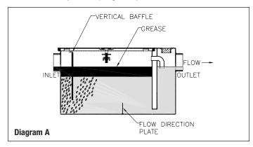
Zurn interceptors have an unobstructed separation chamber permitting the entire baffle to be lifted upward and removed. This provides for fast, easy cleaning which minimizes the amount of time the lid is off and the contents are exposed to the environment.
