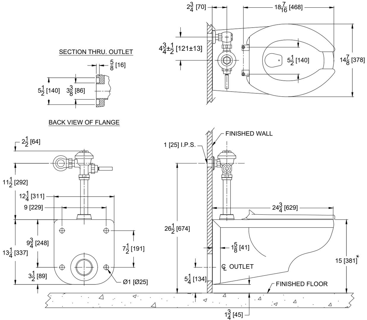
\*NOTE: For ADA compliance, top of seat height should be installed at 17" [431mm] -19" [482mm] from finished floor.
