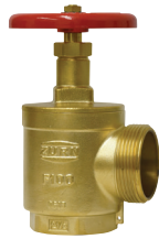
F100 1-1/2", 2-1/2" Inlet: FNPT or Grooved Outlet: NHT or FNPT Option: Special Thread
